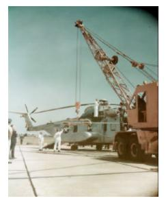
While crew 2 was removing the tail rotor blades and boxing them, mount bolts and rotor-head sling went into the blade shipping box for safe shipment. The first crew's blade bolt remover/installer connected the rotor head sling to the crane as it was jacked up.
