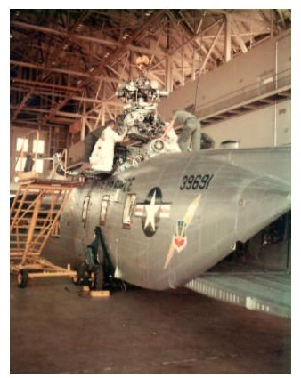
Sikorsky's first attempt to helicopter was load the made with the engines and doghouse cowl installed and there wasn't enough overhead clearance. After these items were removed the second try went fine. The first fuselage was moved to the C-133 front bulkhead using the aircraft interior winch, hooked to front gear. Blades were stored inside the fuselage. Transmissions were stored behind first helicopter
