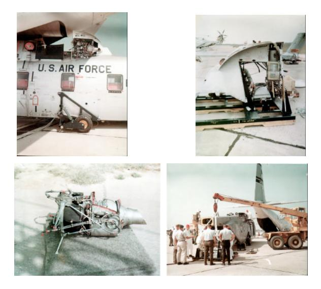
We can now pull the helicopter safely into the C-133. All loading was done with the C-133 loadmaster supervising. With one CH-3 fuselage in place next came the two transmissions on their stands and the two APU storage boxes.
