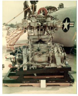
hold down bolts were removed and all the mount bolts were secured in fuselage mount holes. Now crews 1 & 3 worked together to remove the transmission and secure it in its shipping jig.
